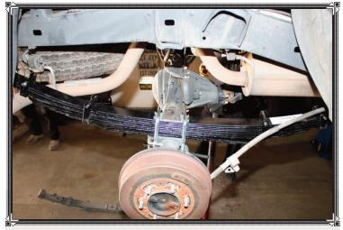
We removed the factory rear leaf springs and bolted in the Deaver Spring Stage II spring packs. The Stage II springs offer approximately 2 inches of additional lift, plus they increase the carrying capacity of our cargo bed by 400-600 pounds.
