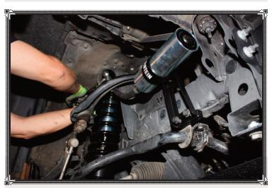
The front B8 8112 shocks include a factory sway bar spacer, which also doubles as the front reservoir mount. Once bolted up, the reservoir is located up and out of harm's way -- clear of any moving parts, and it wont contact the tire at full steering lock.
