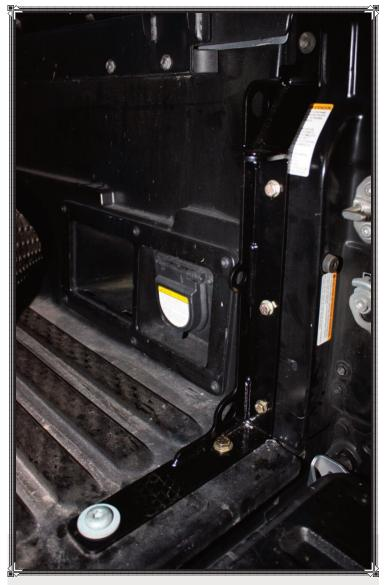
Now that our chassis has been upgraded to heavy-duty levels, we felt that our cargo bed was in need of more support too. So, we bolted up Total Chaos Fabrication's Tacoma Rear Channel Bed Stiffeners, which help reinforce the factory rear bed channels near the tailgate that can fatigue over time with heay off-road use and/or the added weight of items like cargo racks and camper shells.
