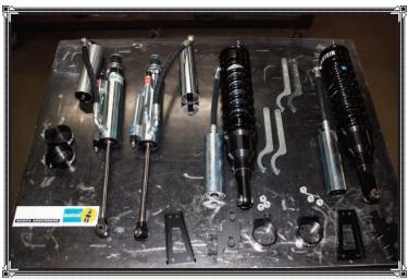
The new Bilstein B8 8100 series shocks are a piece of art, worthy of hanging on a wall in your living room. The front and rear remote reservoirs are 60 mm in length for increased fluid capacity and improved cooling. Built with aerospace-quality components in the USA, the machined aluminum parts ae zinc-coated to resist the harsh elements that Mother Nature is sure to throw at you
