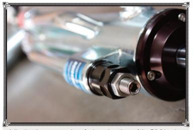
Adjusting the compression of rebound settings of the B8 81--s is as easy as loosening up a jam nut from the bypass adjuster housing and dialing it in with a hex key. There are 10 rotational adjustments for compression and rebound and you can fine-tune your trucks ride with a 1/4, 1/2, or full turn. Turn clockwise to increase damping and counterclockwise to decrease. Then, tighten up the jam nut and you are ready to hit the dirt.
