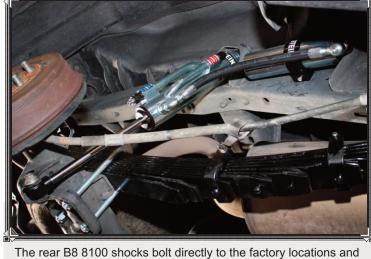
The rear B8 8100 shocks bolt directly to the factory locations and each includes an aluminum anodized reservoir chassis mount, which bolts through existing holes in the frame of the truck. The B8 8100 shocks are specifically designed for the Deaver Spring leaf springs.
