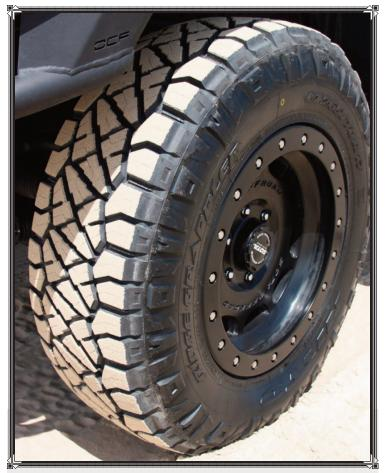
To complement our project, we installed a set of SOTA Offroad D.R.T. 17x8.5-inch wheels with non-beadlock rings. Each D.R.T. aluminum wheel has a 2,600-pound wheel load rating. Finally, we mounted up a set of LT265/70R17 Nitto Tire Ridge Grapplers, which offer a hybrid tread pattern, smackdab in the biddle of a mud-terrain and all-terrain tire. Theaggressive-looking yet quietriding Ridge Grapplers work well in the dirt and deliver a long tread life. **FW**
