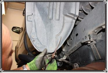
A portion of the rear inner fender liner requires a trimming to accommodate the reservoir. Here, a template is drawn and then cut out.
