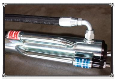
The B8 8100's machined aluminum twin external bypass tubes are absolutely gorgeous and are full adjustable, with multiple compression (in blue) and rebound (in red) settings. The remote-reservoir exit port, in the upper right of the image, helps settle the hard impacts at full compression bypass tube, increases bottoming control and eliminates the need for a hydraulic bumpstop.
