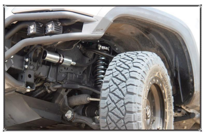
The rear B8 8100 (bypass) shocks are also position-sensitive damped and look like they came off a Baja Trophy Truck. The twin-tube external bypass design features "incremental flow" bypass adjusters, allowing you to adjust the ride of your truck depending on the amount of gear and added weight loaded in the bed. When the going gets rough with unexpected G-outs, the shock utilizes a bottom hose remotereservoir exit port for increased compression control at full
