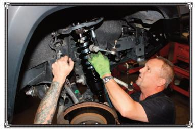
After unbolting the front spindle from the upper control arm, we removed the factory shocks and then installed the B8 8100 shocks using the factory hardware. For our vehicle configuration, the B8 8112s were set from the factory with 1.4 inches of lift. When the truck is unloaded, the rear end sits slightly higher than the front; with a full load of gear in our bed, the truck sits level.
