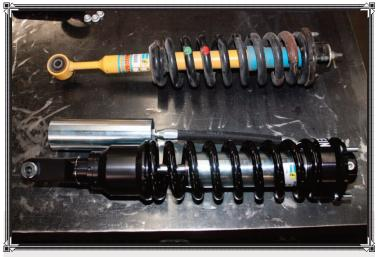
Side by side, you can see how much beefier the B8 8100 (ZoneControl CR) shocks are compared to the factory Bilstein shocks that were included on our Tacoma. The remote reservoir allows for a lot more fluid to cycle through the shock body, while keeping oil temps cooler and decreasing the chances of bottoming out on harsh bumps.
